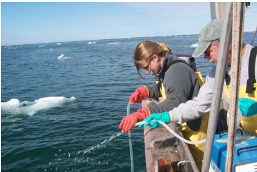
Pumping up clean water samples using a peristaltic pump.
